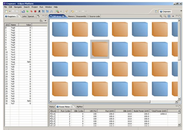
Such systems offer enormous benefits, particularly in their ability to be reprogrammed to do a variety of tasks. The *Cmpware* toolkit provides a powerful environment for the programming and modeling of multicore and multiprocessor architectures, giving previously unavailable visibility into the details of the system state and performance. Such visibility into the internal working of a multiprocessor device is invaluable in designing, analyzing, programming and debugging such systems.
